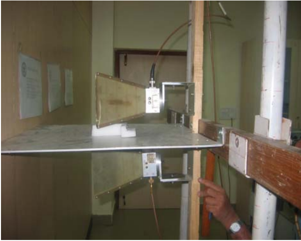
Fig. 1: Bi Static pair of Horn Antenna placed on one side of wall
